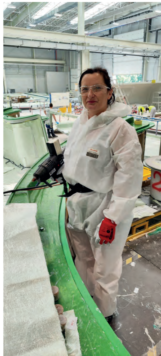
Operators using hot melt adhesive guns during the lamination process at our in factory in Poland
